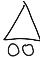
Figure 2. A sketched example of a simple roller support
